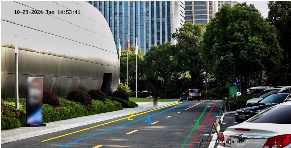
Figure 6-8 Recommended Driving Routes for Force Auto Calibration
